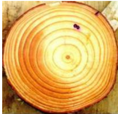
Figure 4.1 : Compression wood in leaning stems, moderate.
