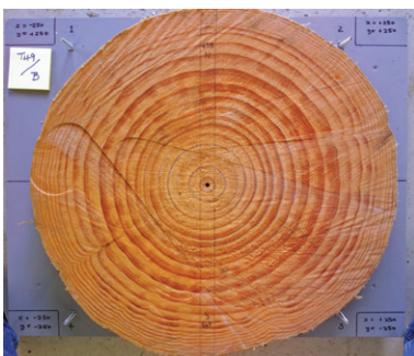
Figure 3 Compression wood all round the stem cross-section.
