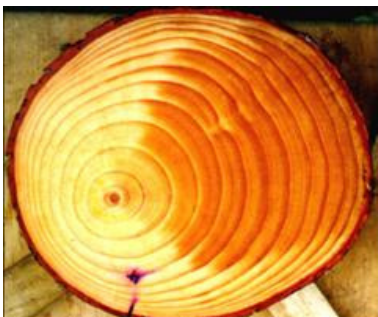
Figure 4 : Compression wood in leaning stems, severe,.
