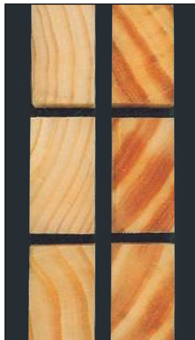
Figure 5 :Normal wood (Left) and Compression Wood (right)
