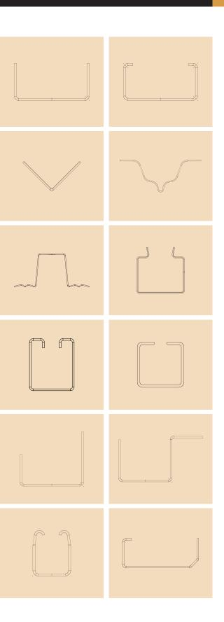
**Rollforming Services** offer a custom roll forming service where we can tool up a machine to do limited runs of your custom profile as you need it. This allows you to design a product exact fit for purpose, therefore reducing rework or wastage experienced when using off the shelf angles and channels.
